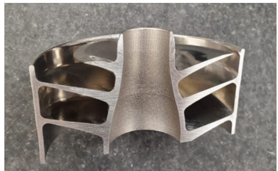
A supercritical CO 2 pump inducer designed by Barber-Nichols. Turbomachinery is an excellent candidate for VELO 3D 's support-less process. This is one of the most challenging parts to machine, and the ability to 3D print these without support structures makes them a viable and profitable part for AM. Source: Barber-Nichols
