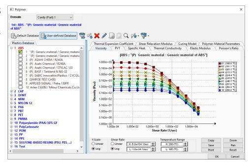
The first step to creating a custom material would be to obtain the proper data. Sometimes the material manufacturers will supply the data upon request. Another method would be to send the material samples to a lab and have them tested for the data.
