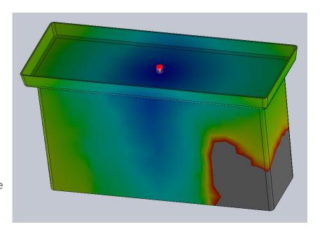
\*\* Warning C1002 \*\* Pressure has reached the max. inject pressure 100.0 MPa !! Error C2005 !! A Short-Shot has occurred during the Flow Process The flow rate is less than 0.010000 of initial flow rate. Inlet Gate Pres.= 100.00 Mpa Is too Small
