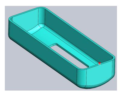
The injection location is where the melted plastic flows from the runner system into the part cavity. Multiple locations can be used but at least one is required to run an analysis.
