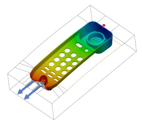
Air traps usually cause molded part defects that range from bubbles in the plastic to burn marks caused by the combustion of the trapped air.
