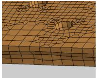
**Automatic mesh** type is the fastest approach and does not require any user input. First, the software creates a curvature-based surface mesh with the size of the elements determined by part dimensions. Next, the software creates a solid mesh from this shell mesh using tetrahedral hybrid elements. If the tetrahedral hybrid approach fails, the software will attempt to create a mesh using orthogonal hexahedral elements. The elements in an orthogonal hexahedral mesh do not curve.
