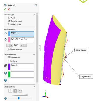
A "Surface Push" was used to create the last deform area.
