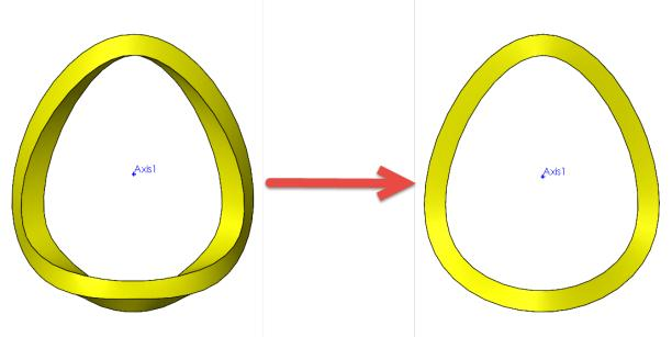
Changing the Profile Twist to "Minimum" did not fix it, so we were able to use the Specify Direction Vector. In this case we used an Axis, but we could have used a plane instead.
