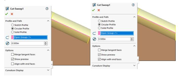
In this case "Align with end faces" extends the cut all the way to the end face.
