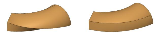
You can also manually adjust the way the profiles come together by using "Show all connectors" from the context menu, then dragging them around. Be aware this isn't as precise but is more of a drag-and-drop-as-close-as-you-can sort of tool.
