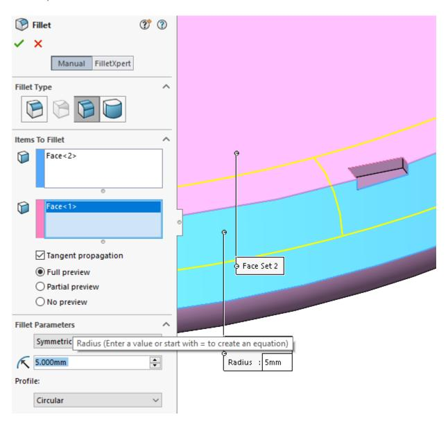
Face Fillets also allow the use of a "Hold Line". This will create a fillet tangent to the selected faces and the radius will be automatically adjusted so the Fillet ends at the Hold Line edge(s).
