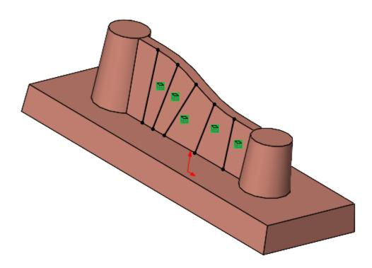
(Another way to preview how the intermediate profiles would rotate is by using face curves in a 3D Sketch: Start a 3D Sketch, turn on Face Curves and select a face.)
