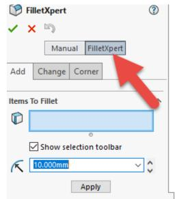
The "Corner" tab allows you to choose between different blend options where three Constant Size Fillets of mixed convexity come together.
