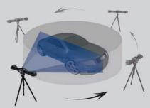
Flexible measurement volume that can be easily and dynamically extended without loss in accuracy or conventional leapfrogs.
